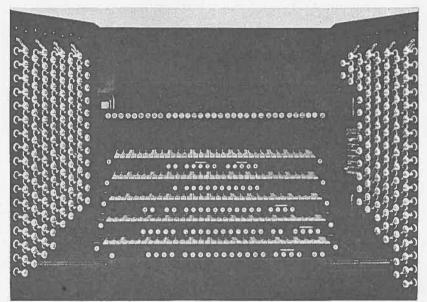
THIS PICTURE shows the new five-This picture shows the new five-manual console of the great organ in the Liverpool Cathedral. This console was installed in 1939 and has several interesting features. The music desk has luminous stops for the couplers. When the fifth manual is not in use it can be lowered, with the couplers. To put on a coupler the organist presses the luminous ivory control and that particular
