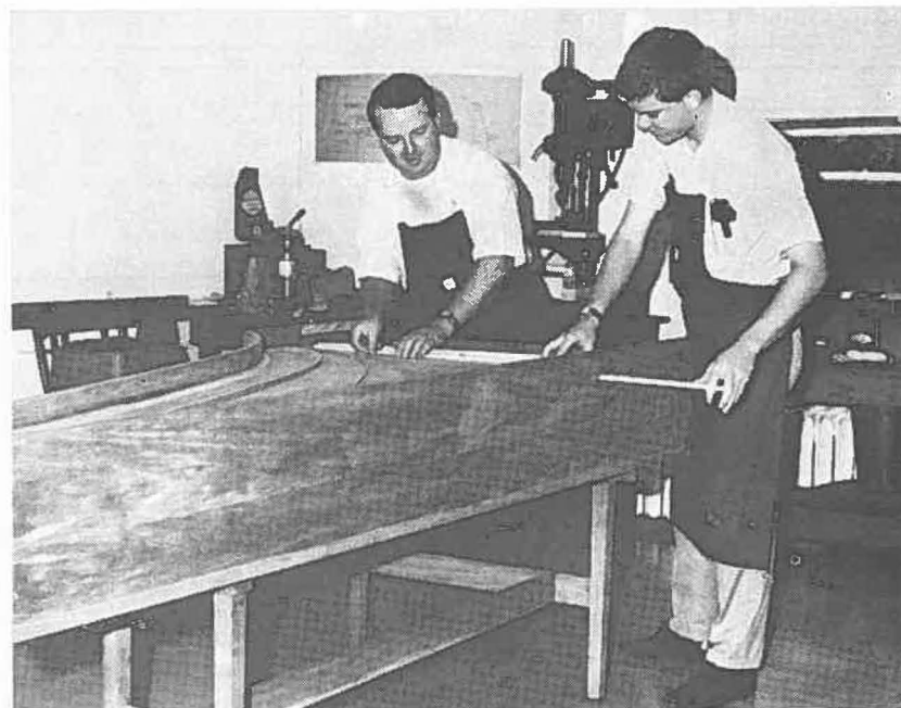
Registers being inserted into the harpsichord frame.
