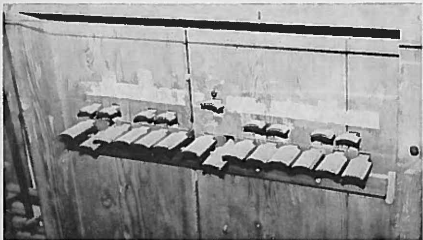
Ex. 5. Keyboard of the Norrlanda organ. Note that B \flat is still grouped with the natural keys at this date. These keys are about twice the width of present-day organ keys.
