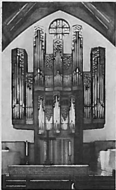
Rudolf Janke: The United Methodist Church of Berea, Berea, Ohio. 3-manual and pedal, mechanical key action, electro-pneumatic stop action, separate hinged bellows for each manual division, swimmer bellows for pedal division, free-standing case, manual compass 56 notes, pedal compass 32 notes.
