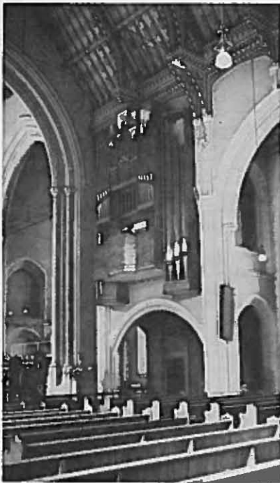
Rushworth and Draper, Ltd.: Ealing Abbey, London, England. 2-manual and pedal, 26 stops, mechanical key action, electric stop action, each division individually encased in polished oak, manual compass 56 notes, pedal compass 30 notes.
