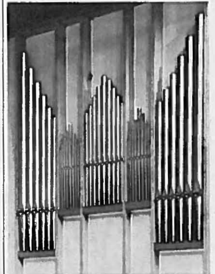
Gress-Miles Organ Company: First Congregational Church, DeKalb, Illinois. 2 Manuals, 25 Ranks; all-electric action. Unison couplers only, except Octaves Graves (Swell) which itself couples to Great.
