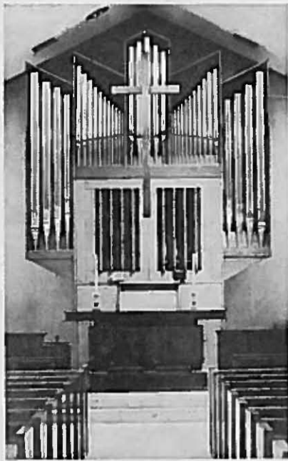
First United Methodist Church, Canton, TX: built by Roy Redman, Fort Worth, Texas. 2-manual and pedal, mechanical key and stop action, free-standing case of mahogany, mechanical swell shades. Wind pressures 2 1/4" (Great), 2" (Swell), and 2 3/4" (Pedal). Dedicated May 13, 1975.
