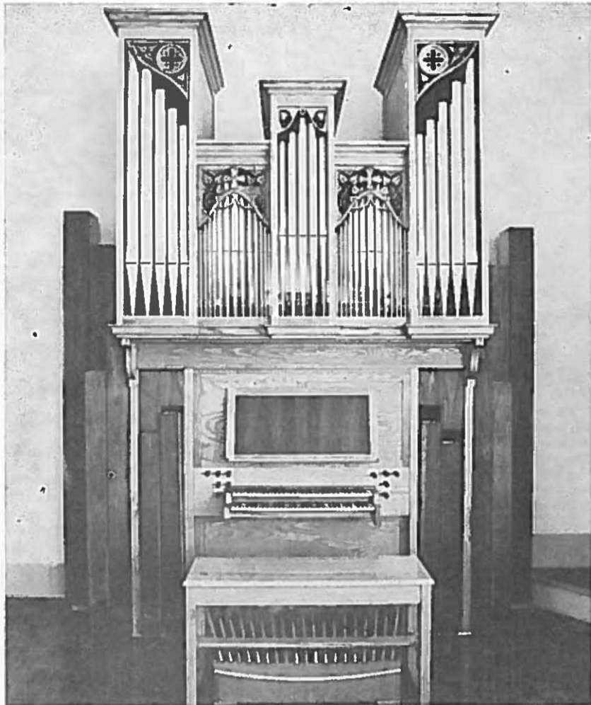
Unity Presbyterian Church Organ by Ralph Blakely Denver, North Carolina Davidson, North Carolina, 1979 Dedication recitalist: Wilmer Hayden Welsh Two manuals and pedal, 61/32 — 10 ranks Mechanical key and stop action
