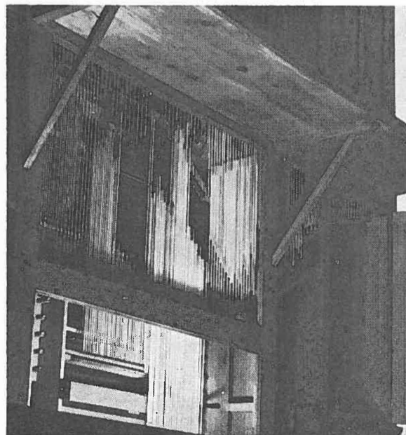
Left: back of case, showing manual and pedal trackers and rollerboard. Above: pallet box and pallets.
