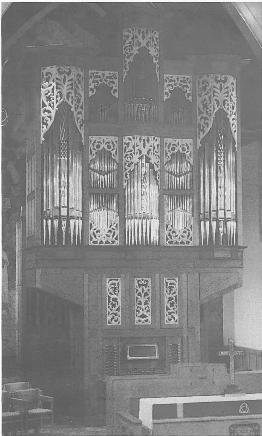
The Noack Organ Co., Inc., Georgetown, MA, has built a large 3-manual organ for Grace Episcopal Church, Grand Rapids, MI. Casework is of solid white oak. The carvings were designed and carved by James Lohman. John Hamersma is organist-choirmaster of the church. A dedicatory recital was played on September 20 by Huw Lewis.
