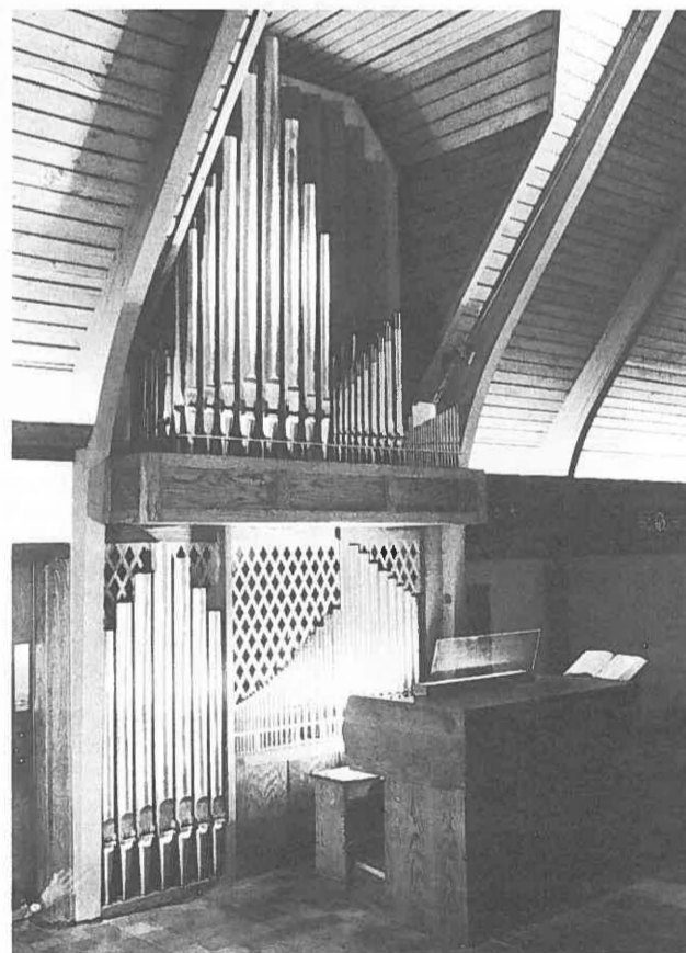
St. Alban's Episcopal Church Cape Elizabeth, Maine 3 Manuals, 25 Ranks, Mechanical Action Opus 88
