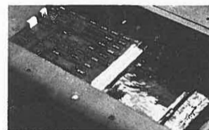
Automatic wave soldering does in seconds what once took many hours by hand, with more uniform connections.
