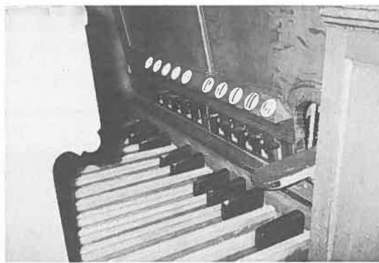
Lower portion of keydesk at Olten (Kuhn, 1880), featuring combination pedals and balanced swell pedal
