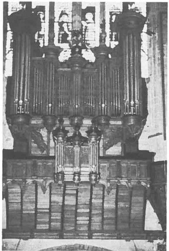
Bourges Cathedral, France. Total restoration by Kern of Strasbourg in 1985 included attached console, mechanical stop action and 3 ventill pedals as the only registration aids.
