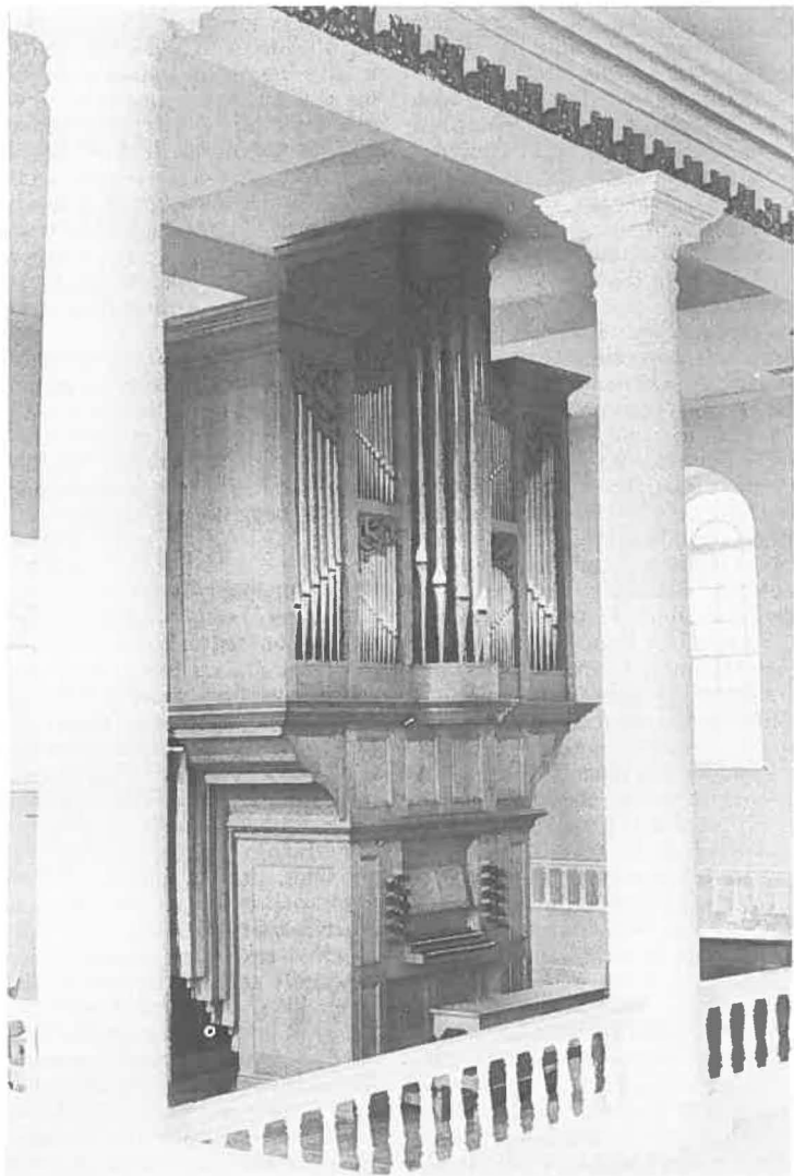
Beaufort, SC (USA). Taylor and Boody Organbuilders, Staunton, VA. Op. 11. Mechanical key and stop action, compass C-e''', C-e', Kirnberger III temperament, metal pipes of hammered lead-tin alloys, case of solid white oak.
