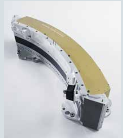
Figure 2: The new Stellar Detector as it is implemented in the CT scanner.
